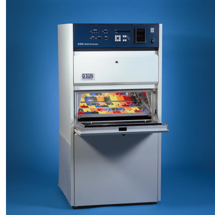
Xenon arc chambers reproduce the full spectrum of sunlight and are generally recommended for testing color change and fade. Optical filters can be used to isolate the Daylight spectrum or Sunlight-Through-Window Glass. Photo courtesy of Q-Panel Lab Products.
